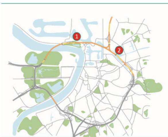
Figure 13: The Oosterweel link, completing the unfinished Ring Road with a new set of tunnels and replacing the current Ring Road Viaduct by tunnels and open trenches to be covered over time
