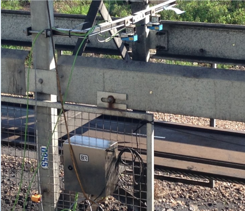
Camera mounted to capture belt staple
