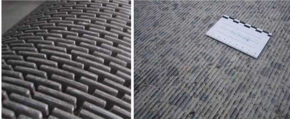
Picture 2) left (a) grinding head, right (b) typical diamond ground texture
