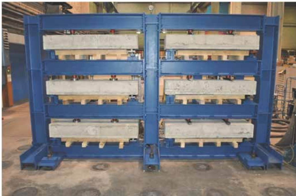
Picture 4) Test setup for simultaneous tests on six large concrete beams
