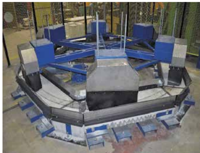
Picture 9) Test setup for simultaneous tests on six large concrete beams with sodium chloride solution applied on top
